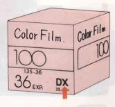
This camera automatically sets the ISO film speed of DX-coded film when it is loaded into the film chamber. Therefore, you are recommended to use only DX-coded film in this camera. (If non-DX film is loaded the camera will automatically set the film speed to 100, whatever film speed it may have; in other words, the only non-DX film usable for this camera is one with ISO 100.)
